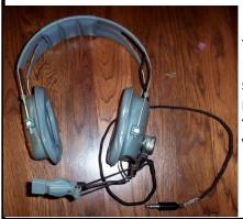
The headsets were common for both front-end and back-end crews. Headsets were plugged in to the airborne interphone communications system (AN/AIC-10) advanced intercom system that permitted hot-mike inter-cockpit communications and a Private intercom capability for back-end operator crew members and the navigator. This system was stalled in all EC-47 aircraft.
